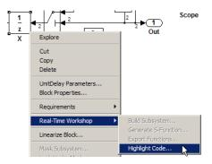
**4** This selection highlights the generated code for the block in the HTML code generation report. The total number of highlighted lines is displayed next to each source file name in the left panel of the HTML report. **Previous** and **Next** buttons help you navigate through the highlighted lines.
