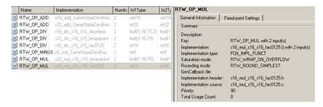
**2** Register a target function library, consisting of one or more replacement tables, using a Simulink s1 customization API.
