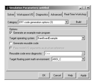
A new group of options supporting use of *code templates*, a powerful and simple technique for customizing generated code, has been added. These options are available in the ERT code templates category of the **Real-Time Workshop** pane of the Simulation Parameters dialog box (see the figure below). Code templates are summarized in "Code Templates for Customizing Generated Code" on page 146.
