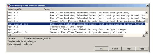
The shared library generated from your model can be dynamically loaded from another application. For example, if you open the demo rtwdemo\_counter, select the ert\_shrlib.tlc target, and generate code, application code similar to the following could be used to dynamically load the generated library file:
